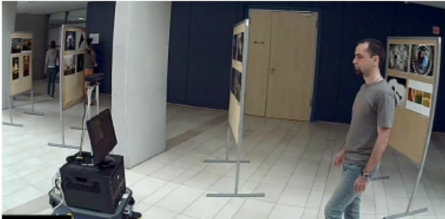
Fig. 1 - Gaze following in the context of joint attention for HRI, using the ROVIS system on a Neobotix MP 500 mobile platform.
