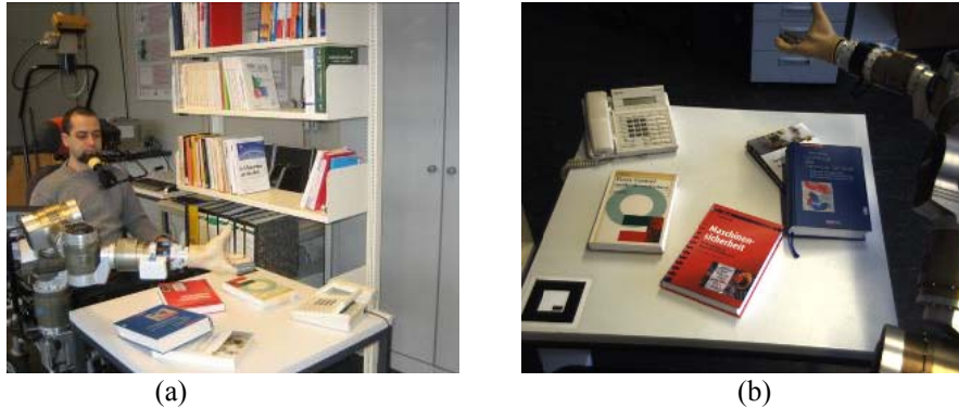
Figure 1: (a) The rehabilitation robot FRIEND operating in a library. (b) A library desk scene imaged by the FRIEND's global camera.
