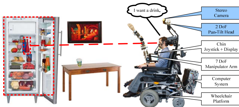
Fig. 1. The rehabilitation robotic system FRIEND operating in complex environment.
